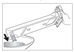
3. Slide the outlet connections in and refit the water reservoir.
